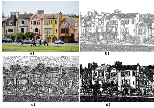
FIGURE 9. a) Original image; b) Canny edge detection; c) GC edge detection with function f_1 ; d) GC edge detection with function f_0
