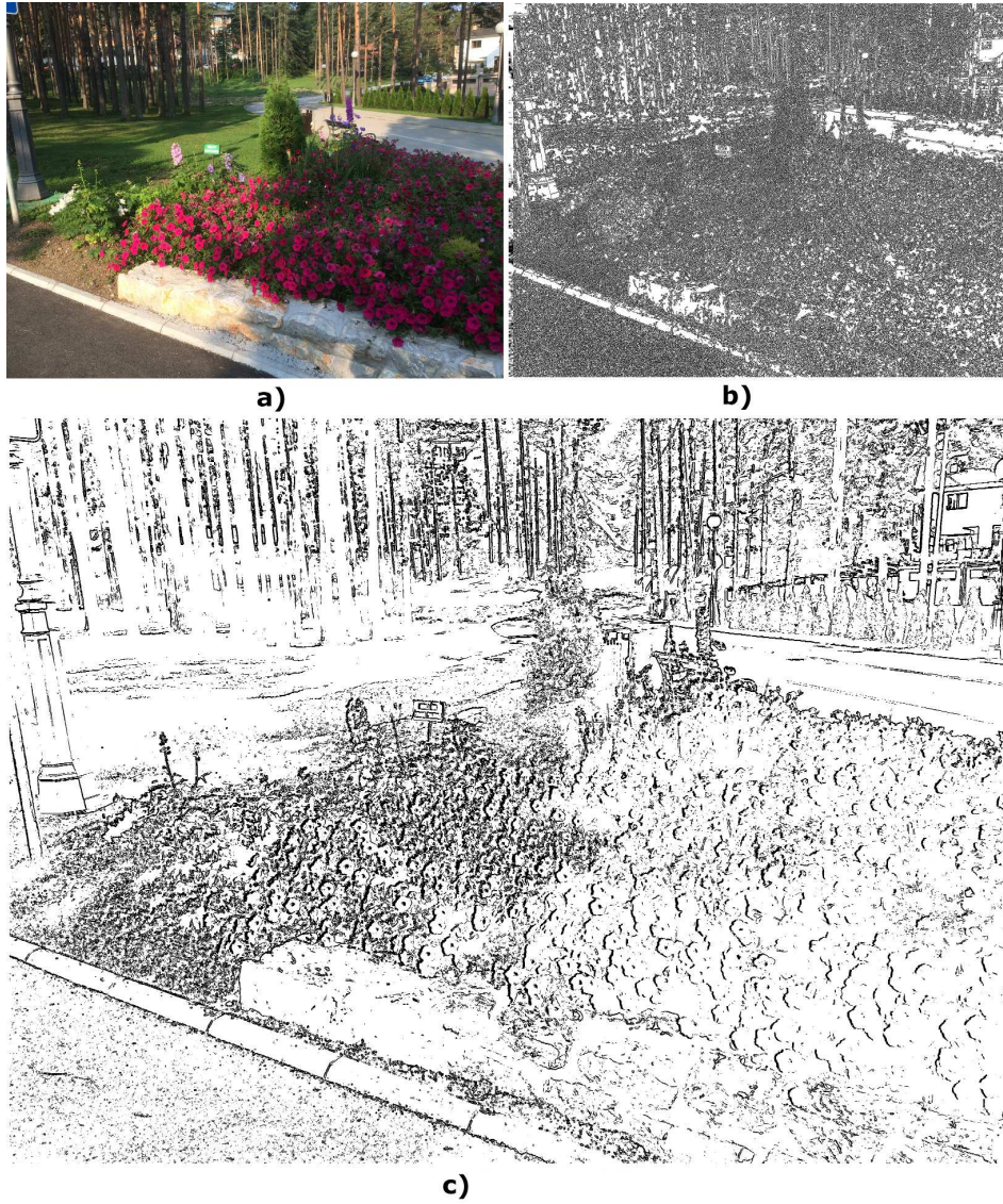
FIGURE 11. a) Original image; b) Canny edge detection; c) GC edge detection with function h_1
