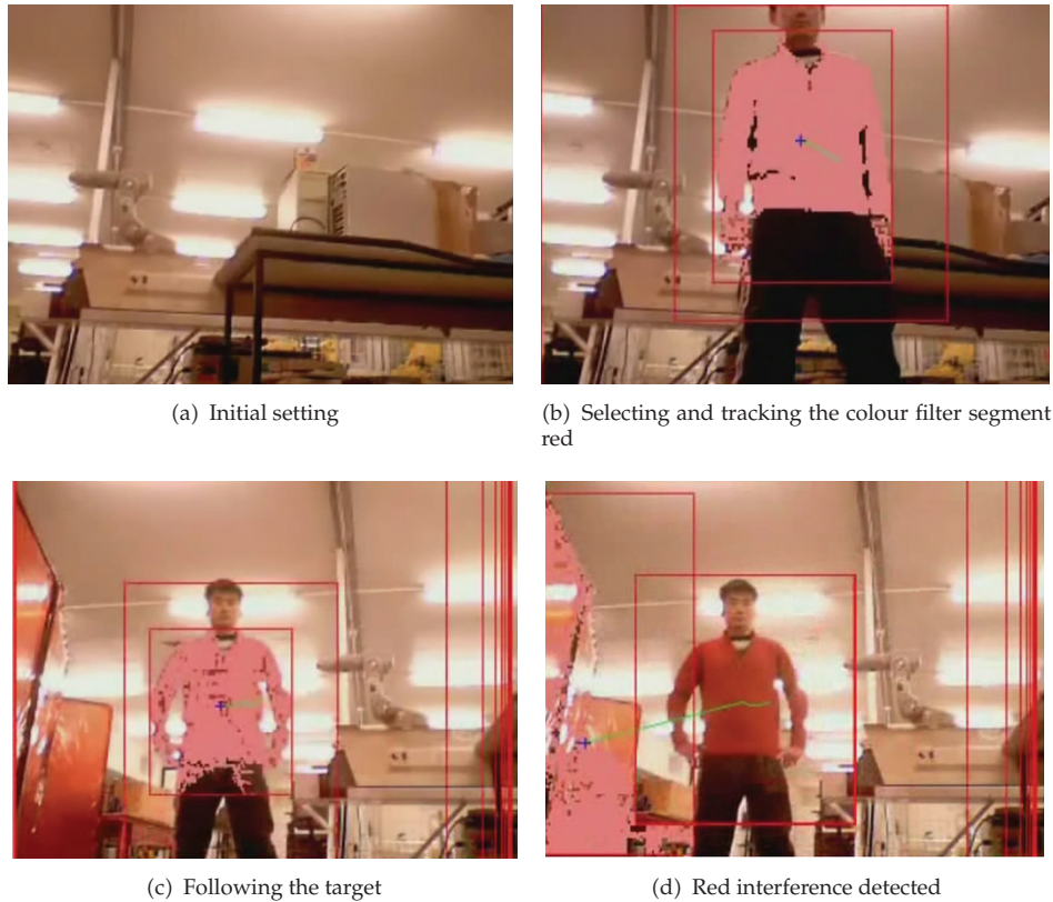
Figure 7: Key video frames of moving object tracking in the complex colour situation part 1.
