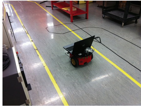
(b) The Pioneer 3 mobile robot
