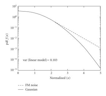
Figure 3.1. FM demodulator output noise pdf (SNR = 12 dB).
