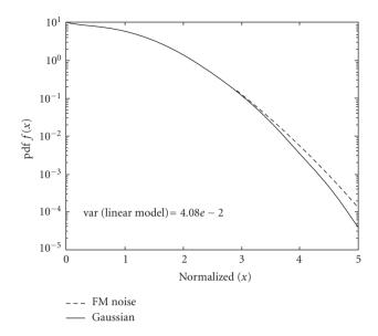
Figure 3.2. FM demodulator output noise pdf (SNR = 20 dB).
