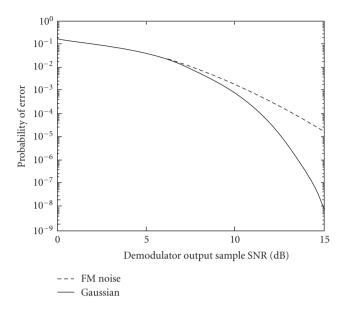
Figure 3.3. Probability of bit error for NRZ signal (SNR  $_i = 12 \text{ dB}$ ).
