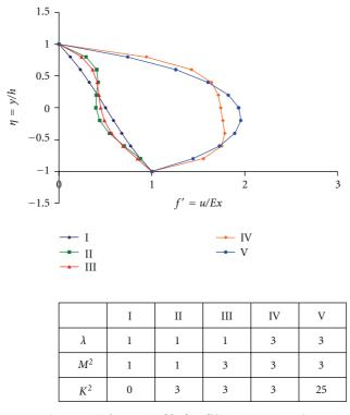
**Figure 3:** Velocity profile for f'(R = 0.1, N = 10).
