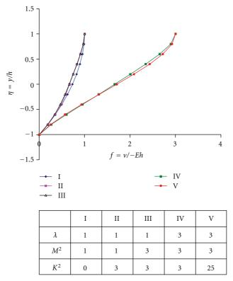
**Figure 2:** Velocity profile for (R = 0.1, N = 10).
