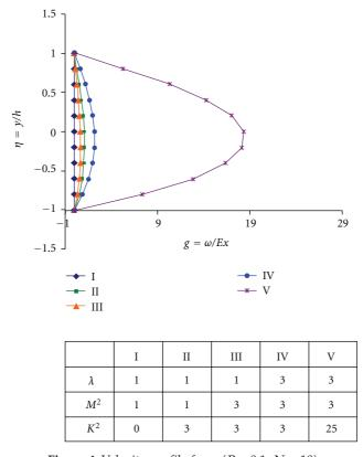
**Figure 4:** Velocity profile for g (R = 0.1, N = 10).
