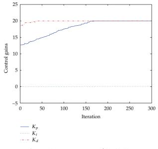
**Figure 3:** Iteration response of  $K_p$ ,  $K_i$ ,  $K_d$ .
