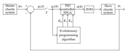
Figure 1: Block diagram of chaos synchronization system.
