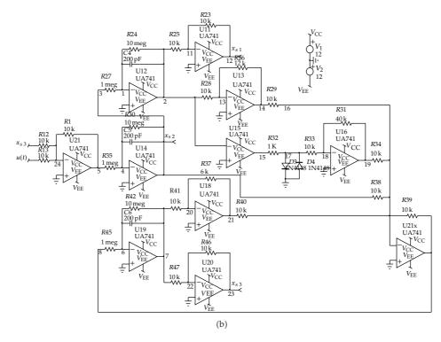
Figure 5: Electronic implementations of Sprott circuits. (a) master system; (b) slave system.
