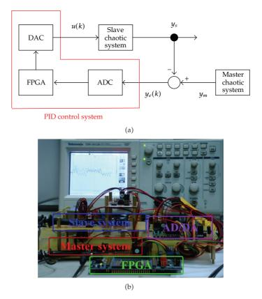
Figure 6: The Black diagram (a) and the photograph (b) of the proposed chaos synchronization system.
