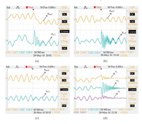
**Figure 7:** Experimental results of synchronization. (a)  $x_{m1}$  versus  $x_{s1}$ . (b)  $x_{m2}$  versus  $x_{s2}$ . (c)  $x_{m3}$  versus  $x_{s3}$ . (d) The error states  $e_1, e_2, e_3$ .
