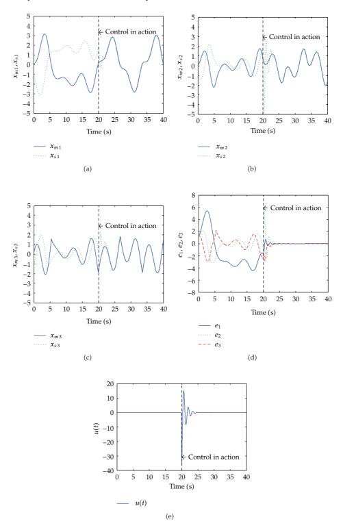
**Figure 4:** Time responses using the EP-based PID controller. (a)  $x_{m1}$  versus  $x_{s1}$ . (b)  $x_{m2}$  versus  $x_{s2}$ . (c)  $x_{m3}$  versus  $x_{s3}$ . (d) The error states  $e_1$ ,  $e_2$ ,  $e_3$ . (e) The control input. (The control u(t) is activated at t = 20 sec.).
