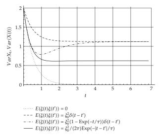
**Figure 1:** The variances as a function of time assuming linear friction. Var(X(0)) = 2, a = 1,  $\xi_0 = 1.5$ ,  $\tau = 0.8$ ,  $t_0 = 0$ .
